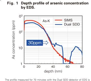
overlaid with the data by SIMS. Detection limit of arsenic dopant is about 1.5×10<sup>16</sup>cm<sup>3</sup> (30 ppm). shown in **Fig. 2**. The boron edge was confirmed to be located at 189 eV as a result of applying the MCR method to the EELS spectrum. The detection limit of boron is about  $5 \times 10^{19}$  cm<sup>-3</sup> (1,000 ppm) as shown in **Fig. 3**.
