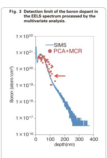
The boron doped sample was measured by STEM-EELS and SIMS. The ALS-MCR method was applied to estimate the detection limit, after noise reduction (PCA), background removal (Power-low model), and multiple scattering removal (Fourier ratio deconvolution).
