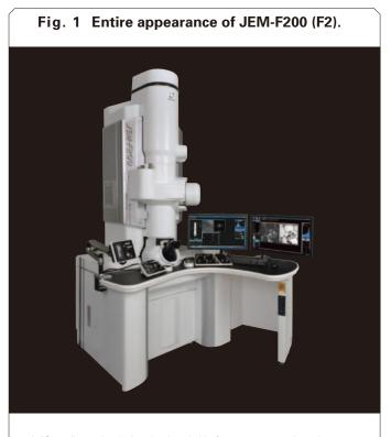
A "Smart" exterior design that is suitable for a next-generation microscope is made by adopting pure white for the base color and metallic silver for the accent color. In addition, the placement of apertures and detectors is optimized to make no protrusion of the microscope units.
