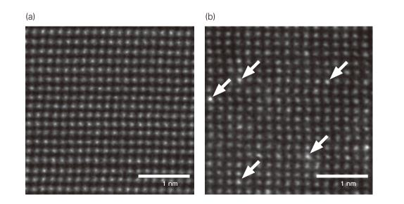
When the incident electron beam propagates along the atomic column which includes another atom, that column shows different contrast compared to the surroundings. (a) No arsenic dopant in the Si substrate. The contrast of any atomic column is the same.
