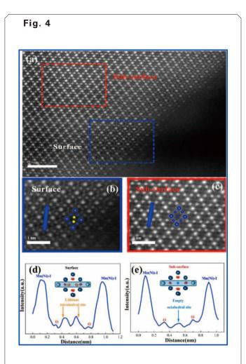
(a) A typical STEM image showing the surface and subsurface regions of the first-charged sample taken with a JEM-ARM200F; (b and c) enlarged regions of the surface and subsurface corresponding to the blue and red boxes in panel (a), respectively; (d and e) line profiles corresponding to the blue lines in panels (b) and (c), respectively. [Schematic lattice structures are overlaid in (b)–(e).] Reproduced from ref. [48].
