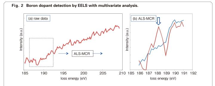
(a) EELS raw data of the Si substrate including boron dopant. There is no edge of boron in the raw data of EELS spectrum from a boron doped sample. The part in the dotted square was analyzed by MCR.
