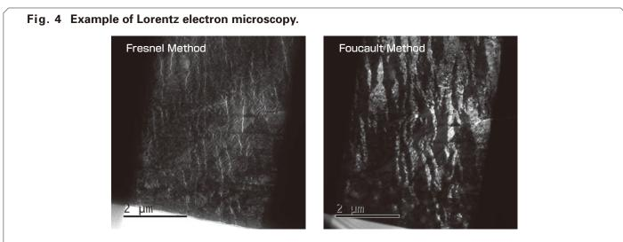
Lorentz electron microscope images (Fresnel method and Foucault method) of Sm<sub>2</sub>Co<sub>17</sub> magnet thinned with a JEOL JIB-4000 Focused Ion Beam System. It is confirmed that nano-scale magnetic domain walls and magnetic domains are clearly imaged with sufficient contrast.
