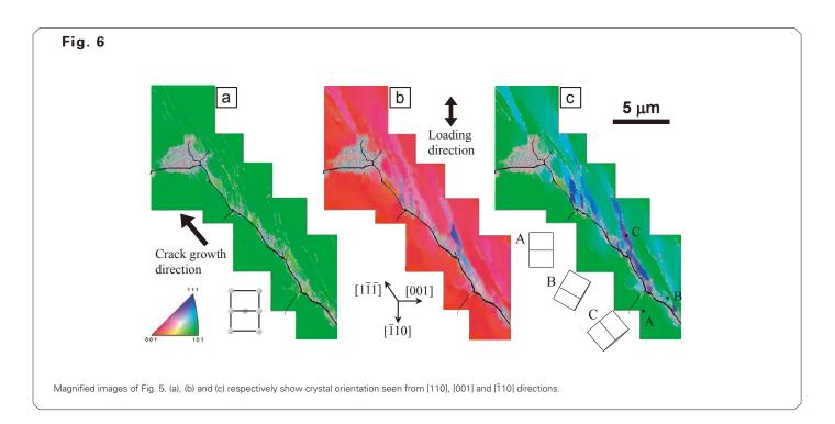
changed by the dislocations emitted from the crack tip in the conjugate slip directions (i.e.  $[1\bar{1}\bar{1}]/[\bar{1}1\bar{1}]$ ). It is then postulated that the present oblique FCG is attributed to the crack tip opening/closing caused by the alternate activation of two slip systems (slip-off mechanism).
