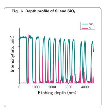
optical thin film was attributed to the existence of elemental Si located at the interface between the  $SiO_2$  and  $TiO_2$  layer. The XPS system of JPS-9030 with Kaufman type ion source makes it possible to measure depth profile data with good depth resolution and keeping chemical state.
