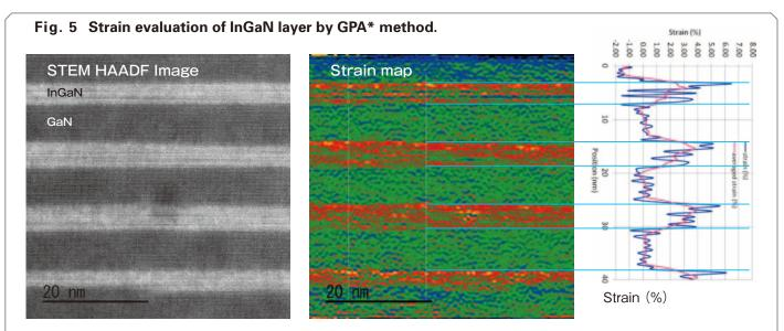
The lattice strain in a local area was visualized by the GPA method which indicates a variation of the lattice spacing directly in the high resolution image of InGaN/GaN layer. The shift of the atomic location due to the addition of In is extracted by comparing the atomic location of pure-GaN. The phase shift is measured and analyzed similar to the electron holography.
