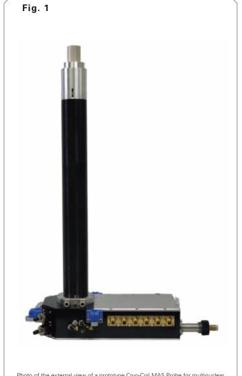
Photo of the external view of a prototype Cryo-Coil MAS Probe for multinuclear measurement.
