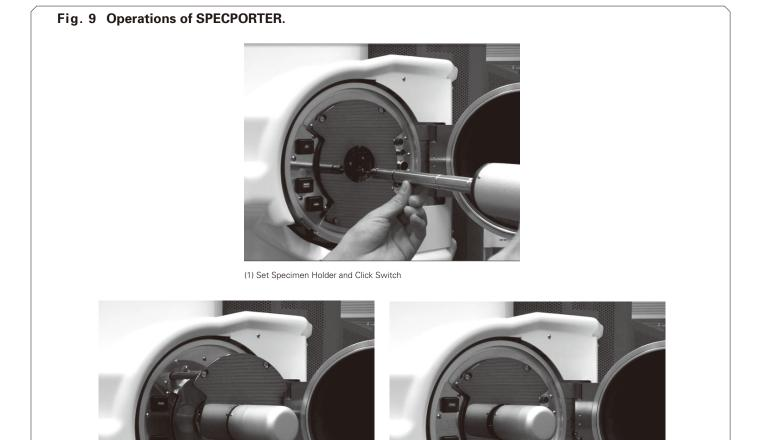
(1) Set a specimen holder at a designated position and click a switch to (2) open the isolation valve with the loading-plate catching the specimen holder and rotating the
