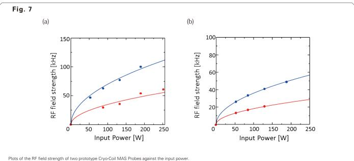
(a) RF field-strength dependence on the input power for <sup>6</sup>Li (with the fifth prototype. Carrier frequency: 88.3 MHz)
