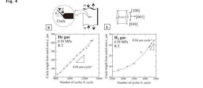
Comparison of growth properties of oblique fatigue cracks in different environments: (a) in helium gas, (b) in hydrogen gas. Material: single crystalline Fe-3.2% Si alloy, stress amplitude: 280 MPa, stress ratio: 0.05, frequency: 1 Hz
