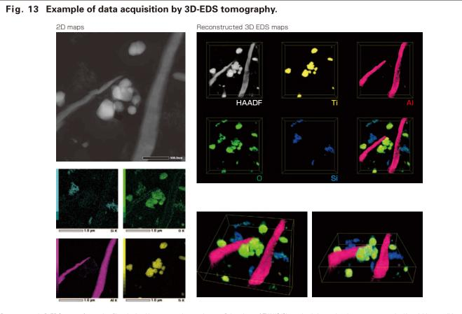
Reconstructed 3D-EDS maps of a coating film obtained by tomography are shown. 3D locations of Ti/Al/O/Si are clearly imaged at the nanometer scale. (Acquisition conditions: Accelerating voltage: 200 kV, EDS: JEOL-made 100 mm<sup>2</sup> SDD, Tilt range: ±60° (in 5° steps), Image acquisition time: 30 seconds per image, 3D reconstruction with 2715 nm × 2715 nm × 559 nm.)
