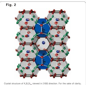
Crystal structure of  $K_2B_2S_{1_{39}}^1$  viewed in [100] direction. For the sake of clarity, splitting of positions (16*i*, 24*k*) is not shown. Green: (Si + B) at 16*i*, red: Si at 24*k* and 6*c*, blue: K at 2*a* and 6*d*. Pentagon-dodecahedra are shown in blue, tetrakaidecahedra in grey. (From Jung *et al.* [10]. Complete atomic coordinates and displacement factors are given there.) Compare the projected structures in Fig. 3!
