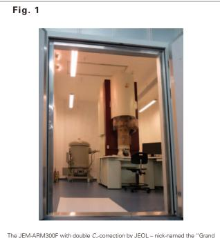
ARM" – in its shielded and air-conditioned booth. This particular booth is placed inside the hall of a new lab building on a non-vibrating fundament.
