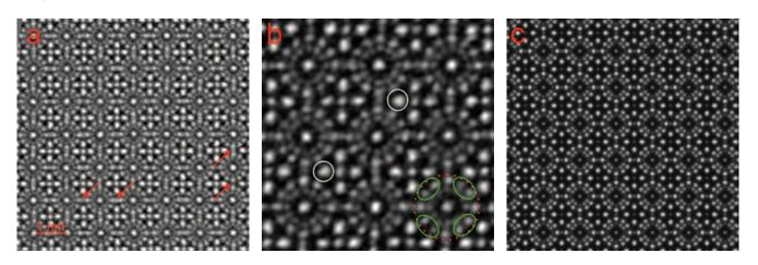
a) Aberration-corrected STEM image (HAADF) of K<sub>7</sub>B<sub>7</sub>Si<sub>38</sub> in [100] orientation. The different potassium occupancies of the 2*a* sites (columns) are revealed better than in TEM imaging. Again, red arrows indicate some exemplary situations.
