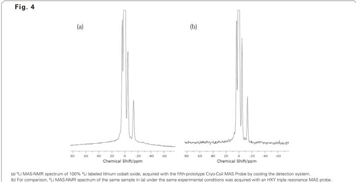
Pulse sequence for the both spectra is Hahn echo (refocus time: 57  $\mu$ s). Input power for the both spectra is 88 W.  $\pi/2$  pulse width is 3.8  $\mu$ s for the spectrum in (a) and 7.0  $\mu$ s for the spectrum in (b).
