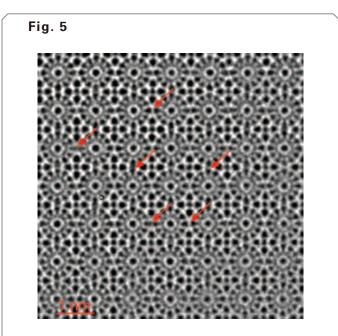
Aberration-corrected TEM image of K,B,Si<sub>30</sub> in [100] orientation. The underfocus regime displays atoms as black. The 2*a* sites, with their statistical 50% potassium occupancy, are situated horizontally and vertically between the rosette-like features. Red arrows indicate some of the many sites where the different occupancies of the sites (more correctly of the respective columns) can be detected immediately. Compare with the simulated images shown in Fig. 4!
