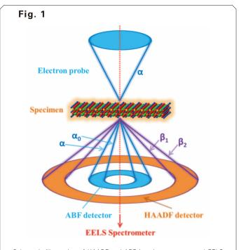
Schematic illustration of HAADF and ABF imaging geometry and EELS collection. A fine electron probe with convergent semi-angle  $\alpha$  is focused to sub-angstrom dimension and scans across the specimen. An HAADF detector at the post column subtends a detecting angle ranging from  $\beta_1$  to  $\beta_2$ ; the ABF detector from  $\alpha_0$  to  $\alpha$ . The EELS spectrometer is located beneath the STEM column.
