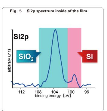
found that Si2p peak had 2 peaks at around 99 eV and 104 eV, which indicates that elemental silicon and silicon dioxide exist respectively. **Figure 6** showed that another depth profile data of Si2p was reconstructed with these 2 components. This figure showed that the component of elemental Si was located at the interface between the SiO<sub>2</sub> layer and TiO<sub>2</sub> layer. From these data and analysis result, it was concluded that the defect in the
