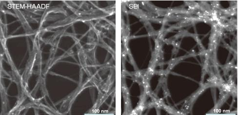
Even at an accelerating voltage of as low as 80 kV, high-quality TEM & STEM-HAADF images and SEI (secondary-electron image) of single-wall carbon nanotube can be observed. The TEM image provides high-resolution information, the STEM-HAADF image shows the Z (atomic-number) contrast, and the SEI reveals the surface information.
