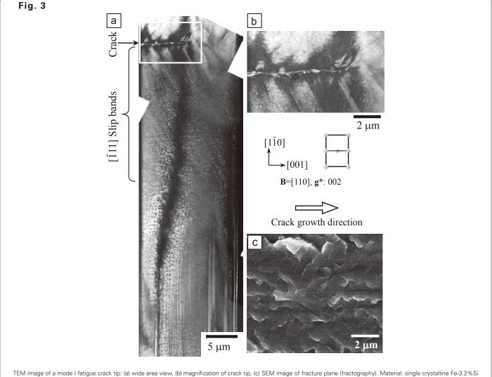
TEM image of a mode I fatigue crack tip: (a) wide area view, (b) magnification of crack tip, (c) SEM image of fracture plane (fractography). Material: single crystalline Fe-3.2%Si alloy, test environment: *hydrogen* gas (0.58 MPa/R.T.), stress amplitude: 280 MPa, stress ratio: 0.05, frequency: 1 Hz,  $\Delta K = 21$  MPam<sup>1/2</sup>, da/dN = 0.25 µm/cycle, V<sub>acc</sub> = 1250 kV, bright field/zero-loss image.
