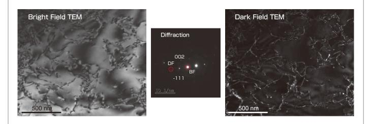
Bright-field & dark-field TEM images are traditionally used for materials analysis. In this example, dislocations in over-aged AI alloy are imaged by an incident electron beam from the [110] direction. Both images reveal the dislocations in a wide field-of-view.
