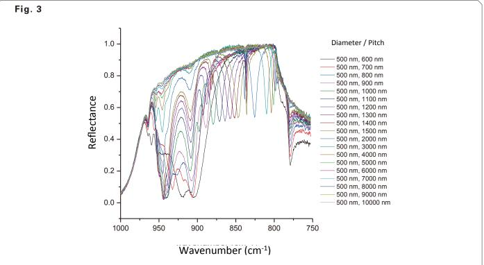
SPhP resonances in nanopillar arrays of 500 nm diameter SiC pillars. By varying the center to center distance (pitch) of the pillars in these arrays, one can precisely tune the spectral positions of these absorptive resonances.
