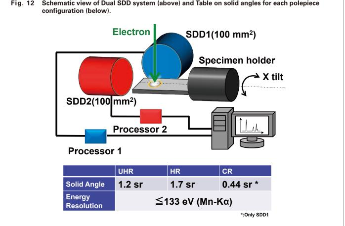
SDD1 is placed at 90 degrees with respect to the specimen holder rod axis, whereas SDD2 is placed along the holder axis. The geometry of SDDs and the specimen holder is optimized to allow larger solid angle for each polepiece configuration, as listed on the table below.
