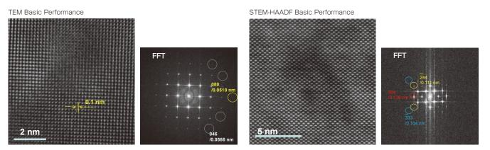
In an FFT pattern of a TEM lattice image obtained from Au (gold) thin foil in the [100] orientation, spots of 0.05 nm (50 pm) are confirmed (second from left). In an FFT pattern of a STEM-HAADF image obtained from a Si (silicon) single crystal in the [110] orientation, spots of 0.1 nm are confirmed (right edge). This result demonstrates high mechanical and electrical stability of F2.
