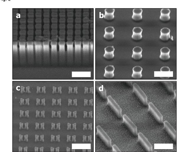
Different designs of phonon polariton nanoantennas fabricated in SiC. All scale bars are 1000 nm. (a) Closely spaced nanopillar array. (b) Widely spaced nanopillar array. (c) Coupled bowties. (d) High aspect ratio cuboids.
