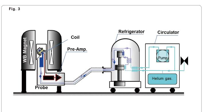
Conceptual diagram of the circulation-type cooling system of the Cryo-Coil MAS Probe. Coloration for each pipe is applied to different temperatures depending on when each pipe reaches a thermal equilibrium state. Blue: Room temperature, Light purple: Medium-low temperature, Dark blue: Ultra-low temperature.
