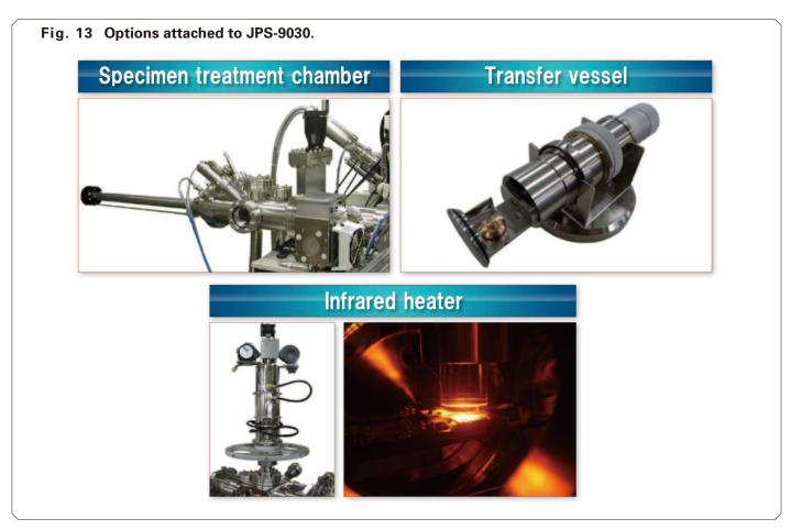
for depth profile analysis of the deeper area in inorganic and organic materials, and also for chemical analysis of the very shallow area with ARXPS or TRXPS measurement. You can choose the many options to expand the potential of XPS analysis. We hope all of you get the good data with our JPS-9030.
