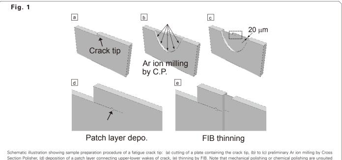
Section Polisher, (d) deposition of a patch layer connecting upper-lower wakes of crack, (e) thinning by FIB. Note that mechanical polishing or chemical polishing are unsuited for the crack tip sample preparation.
