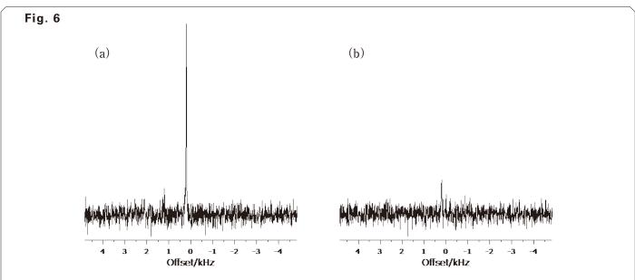
(a) <sup>43</sup>Ca MAS-NMR spectrum of natural abundance calcium oxide, acquired with the sixth-prototype Cryo-Coil MAS Probe, where the temperature of the detection coil is at low temperature (< 17K).
