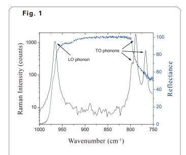
Raman spectra (black line) and reflection spectra (blue line) of un-patterned 6H-SiC. The phonon resonances are seen in the labeled Raman peaks which bound the highly reflective Reststrahlen band.
