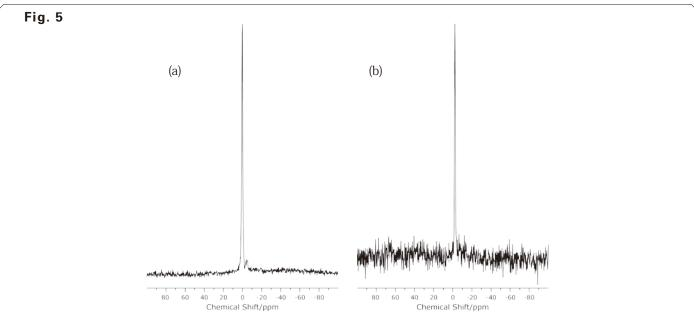
(a) <sup>29</sup>Si MAS-NMR spectrum of natural abundance LTA zeolite, acquired with the fifth-prototype Cryo-Coil MAS Probe.
